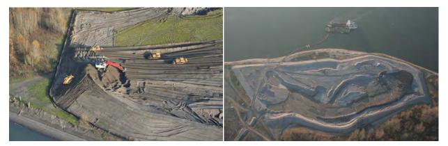
Figure 4: Site preparations and dike building for placement of dredged materials (at Northport).
