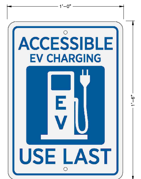
ACCESSIBLE SIGNAGE DETAIL
