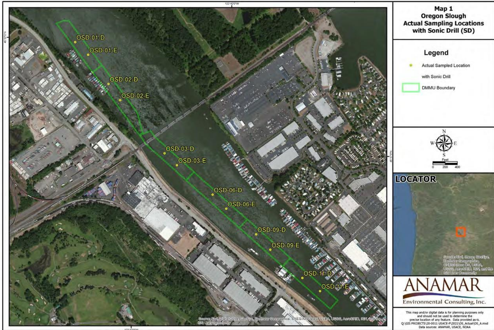
Figure 2. Oregon Slough Downstream shallow draft Federal Navigation Channel, actual sonic drill sample locations (sampled 10-12 May 2021).
