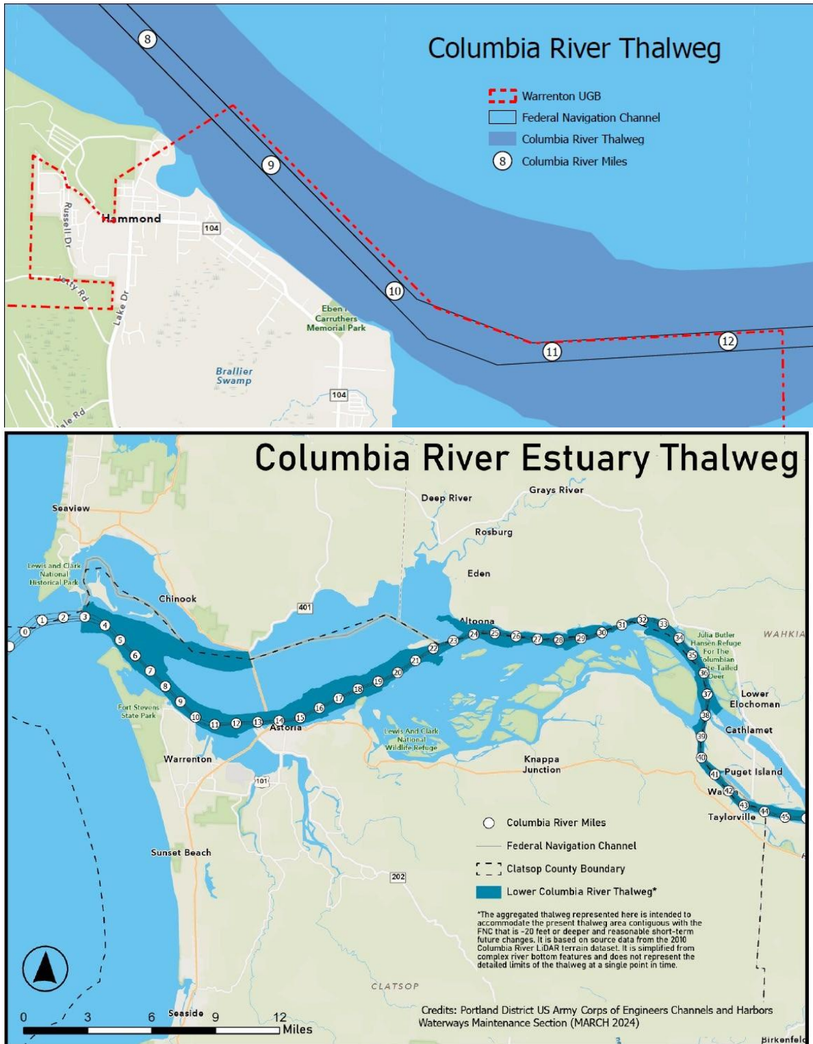
Figure 1 Proposed thalweg for flowlane placement of dredged material in City of Warrenton Urban Growth Boundary and for the whole Columbia River Estuary.
